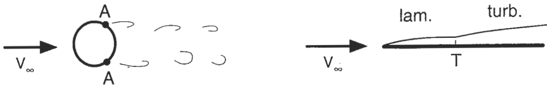
Fig. 27: Pressure drag due to separation (cylinder) and skin-friction drag due to boundary layer (flat plate)
