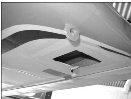
Figure 4. Wingtip's Inertial Platform Hole
