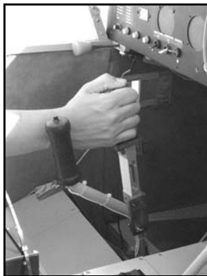
Figure 10. Load cell on command system
